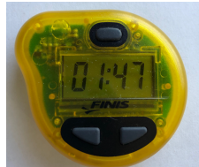
Figure 5. Tempo Trainer Pro (Approximately 4.8 cm in width, 1.4 cm in thickness and 19.5 g in weight)
