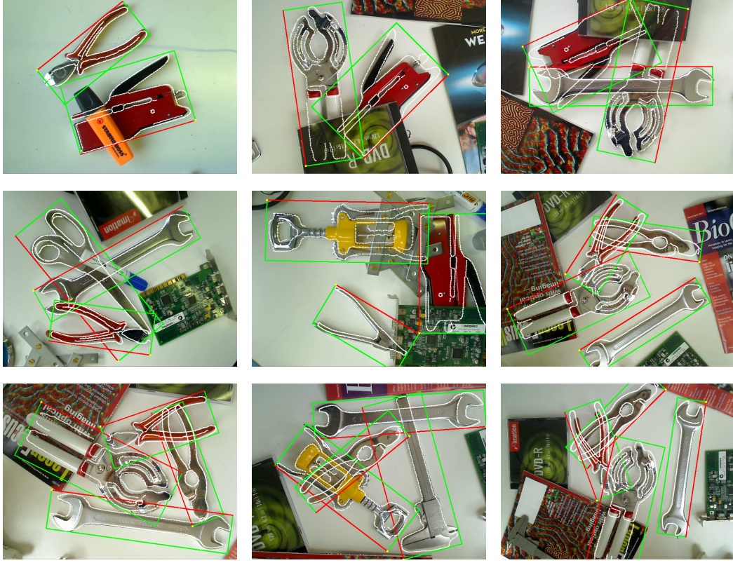
Figure 3.8 Example images of D-Textureless dataset used in Experiment 3. The edges of the objects extracted from the model images (white lines) and the bounding boxes (red and green lines) are drawn based on the detection results by our proposed method.
