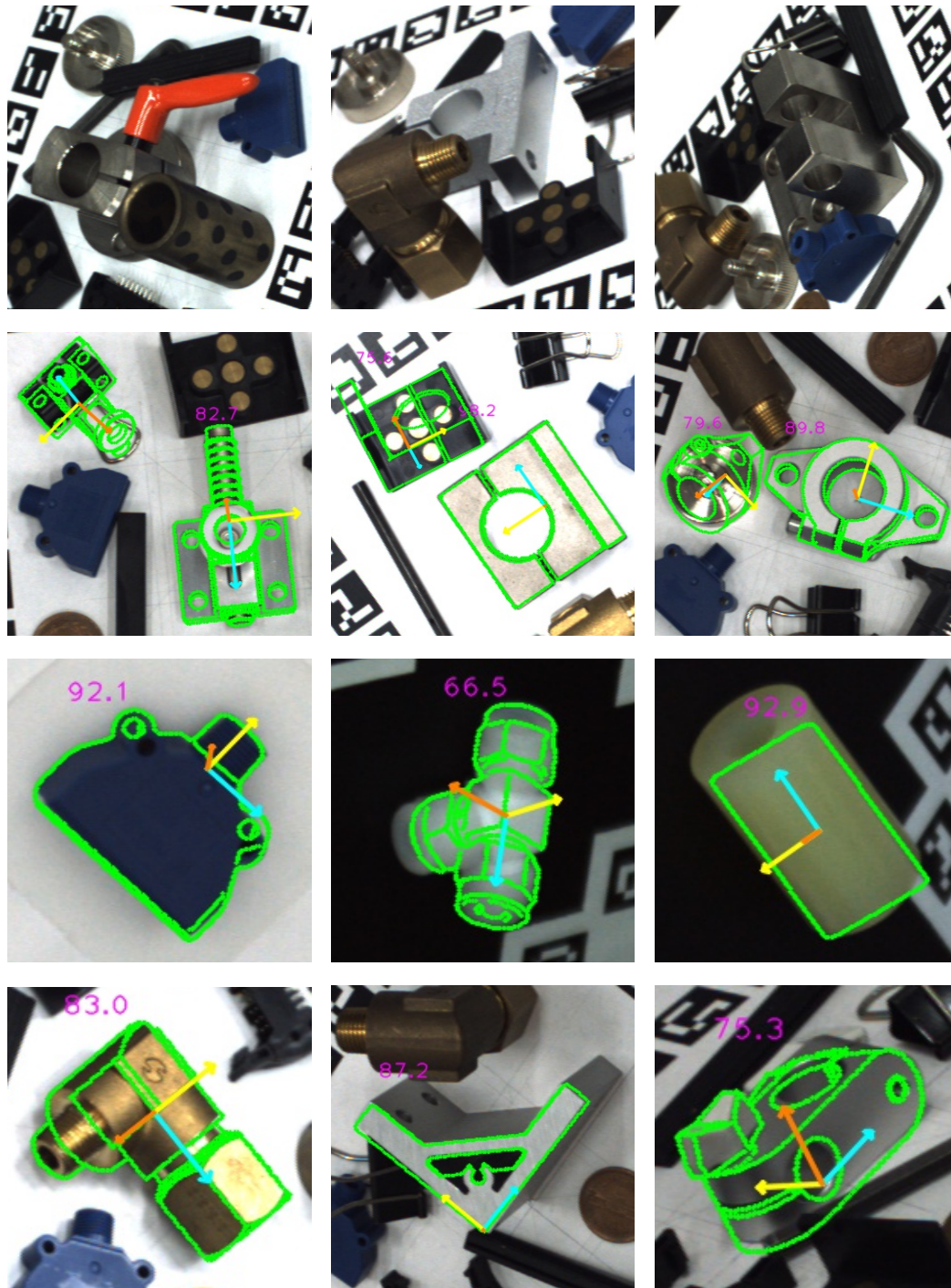
Figure 4.14 Example images of the failure cases of our proposed method. 1st row: Stopper, T-Holder and HingeBase were not recognized due to partial occlusions. 2nd row: There were false positives of SideClamp, T-Holder and Flange due to background clutters. 3rd row: The 3D pose of AirNozzle, FluoroConnector and UrethaneTube were erroneously estimated due to less-visible edges. 4th row: 3D pose estimation of Connector, Bracket and PoleClamp were failed due to partial correspondences. The target objects in 3rd row are from an additional experiment and others are from Mono-6D dataset.
