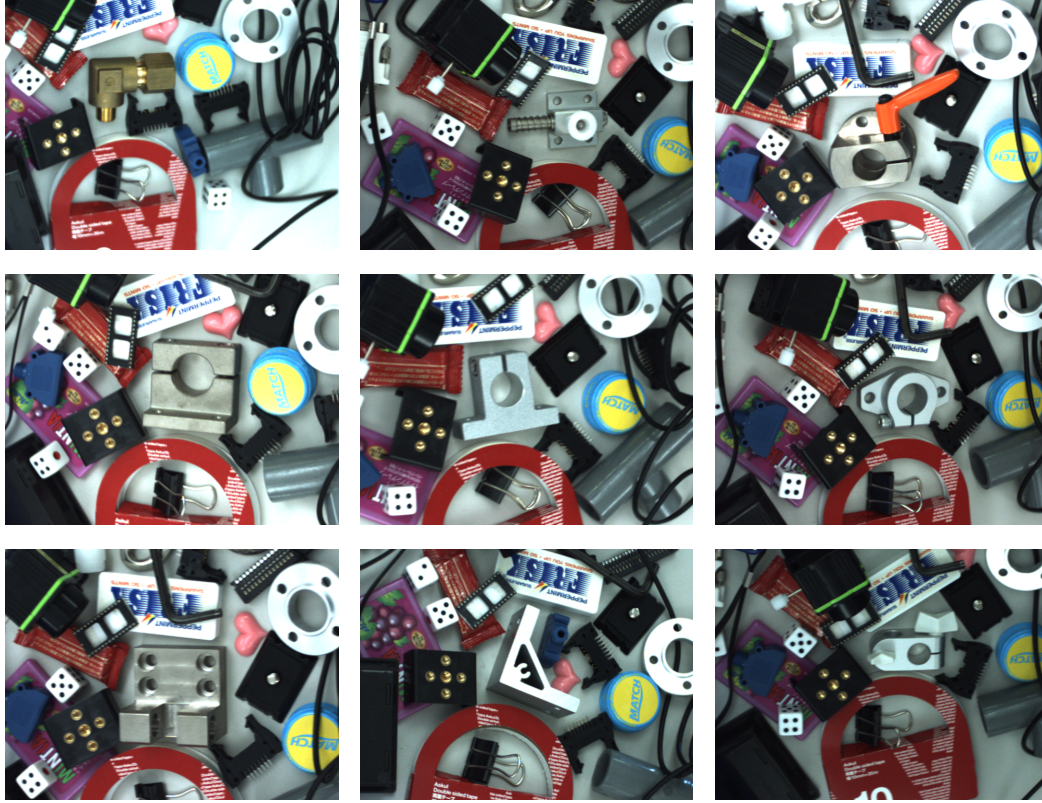
Figure 4.9 Example images used in experiment 1. A target object whose 3D pose is slightly transformed (less than approximately 10 degrees around X/Y/Z axes) is captured under background clutters. Nine kinds of texture-less objects are tested. Top: Connector, SideClamp and Stopper. Middle: L-Holder, T-Holder and Flange. Bottom: HingeBase, Bracket and PoleClamp.
