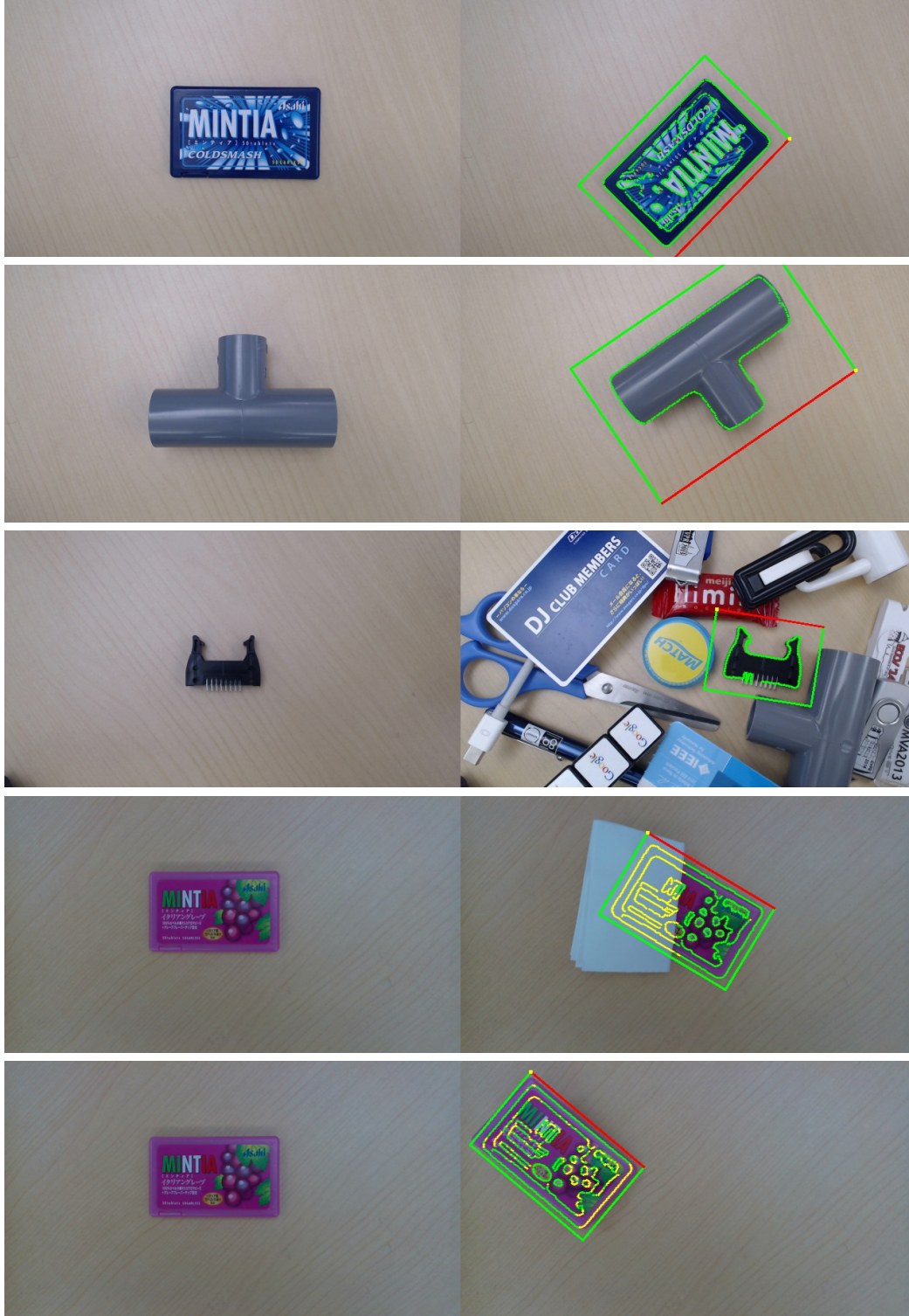
Figure 2.1 Detection results of our global descriptor based method presented in Chapter 3. Top row: A textured package on a simple background. 2nd row: A texture-less pipe on a simple background. 3rd row: A texture-less connector on a cluttered background. 4th row: An occluded package. 5th row: A textured package with perspective distortion. The left images are models and the right images are the detection results where the bounding boxes and extracted edge from the models are drawn. The yellow dots represent the feature points whose correspondences are not found in the input images.
