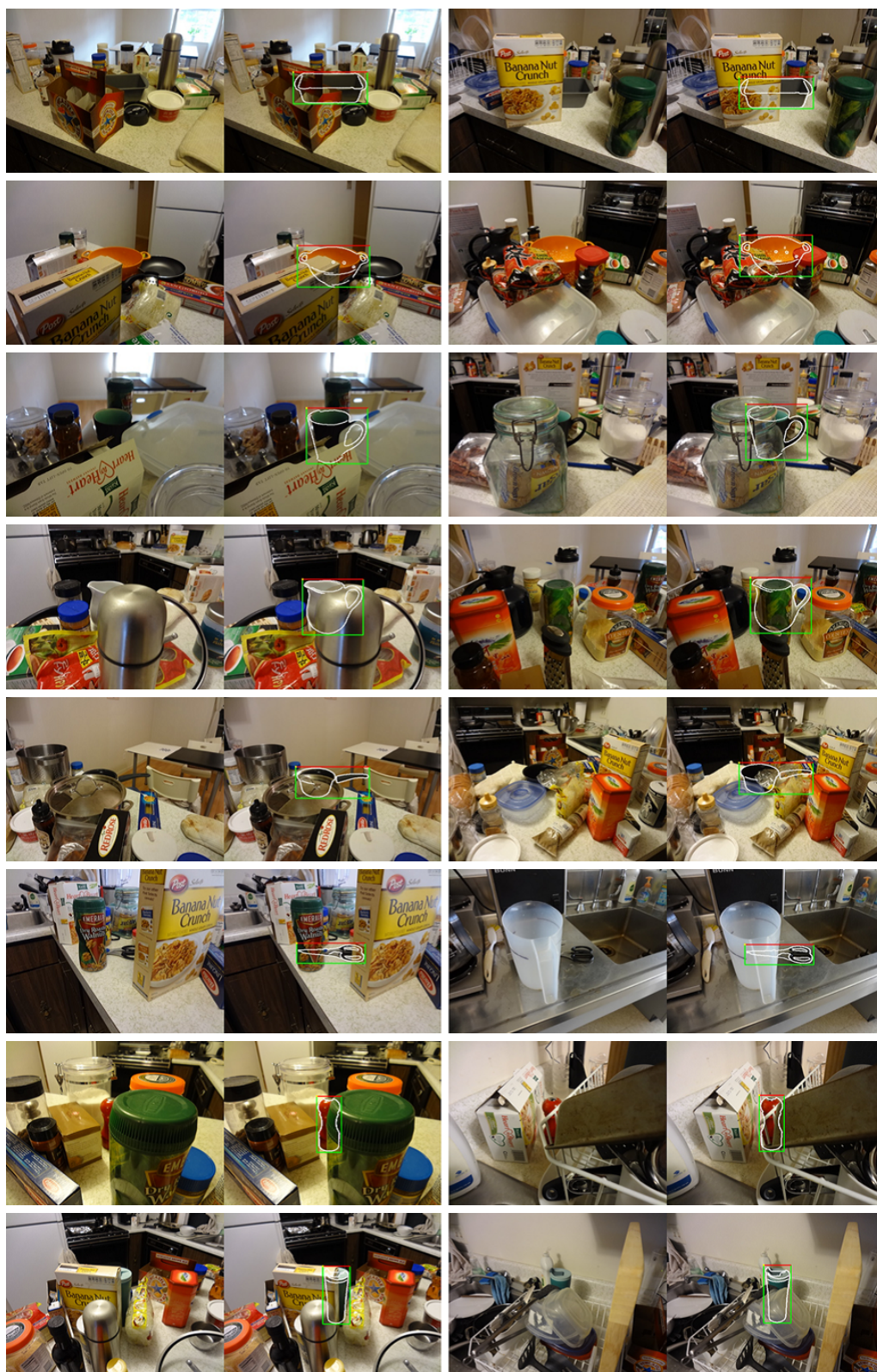
Figure 3.11 Examples of test images from CMU_KO8 dataset (single-view). In each panel, the left is an input image and the right is result image where the bounding box and matched model edge points detected by our algorithm are drawn.
