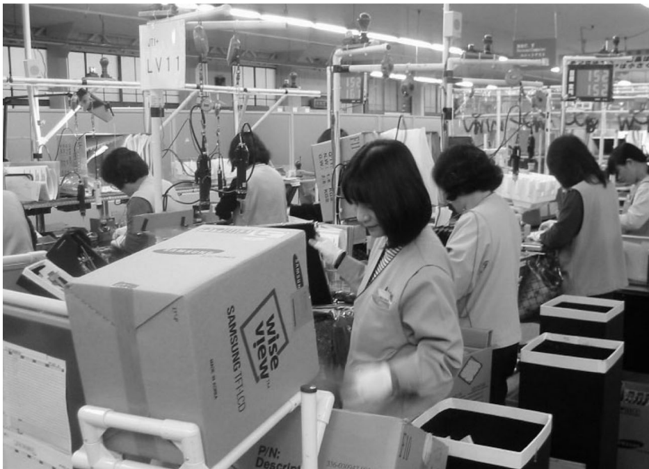
Figure 1 A small workgroup (what is referred to as "cellular manufacturing") in Japan where a workgroup of four operators assemble lap-tops. Note the display in the top right corner which shows the workgroups planned and performed production at this exact moment. Unlike Swedish production systems with parallel product flows in Japan it is obvious that the operators must have information about the workgroups' current performance in relation to the production plan.
