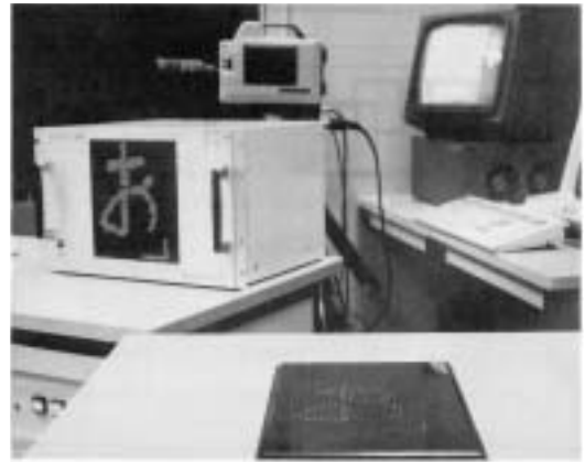
Fig. 8 Hiragana "O" presented on CRT, LED, and Tactile Graphic Display. 図10 自己保持型触覚ディスプレイ
